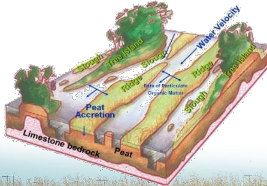
TYPICAL CROSS SECTION OF THE EVERGLADES - RIDGE AND SLOUGH TOPOGRAPHY -
